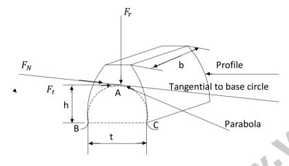
The tangential component  $F_t$  induces a bending stress which tends to break the tooth. The radial component  $F_r$  induces compressive stress of relatively small magnitude therefore its effect on the tooth may be neglected. Hence the bending stress is used as the basis for design calculations.
