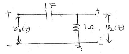
Assume the sampling rate  $f_s = f_0$  where  $f_0$  is the cut off frequency of the analog filter shown.
