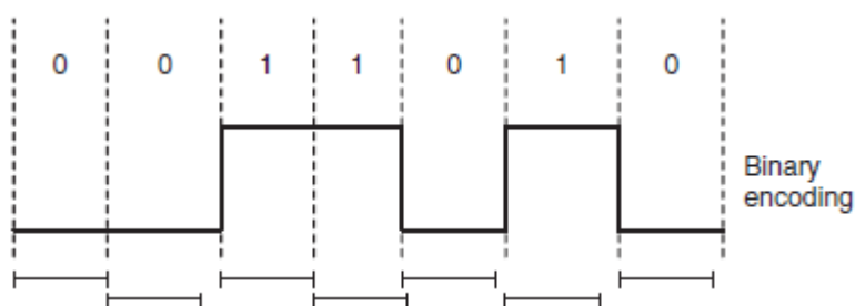
Figure 4.12 Due to physical properties the signals are not always the same length at the receiver (jitter).
